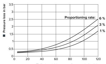
Extinguishing water flow rate in % of the maximum permitted flow rate of the particular FireDos proportioner
