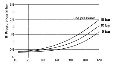
Extinguishing water flow rate in % of the maximum permitted flow rate of the particular FireDos proportioner
